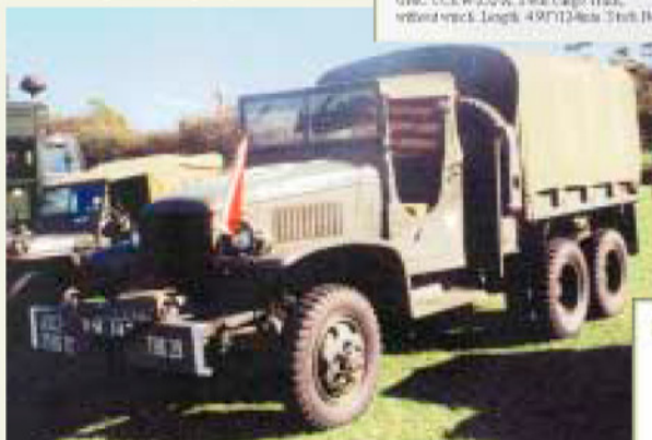
GMC CCEW 213-A, 1 1/2 Ton Cargo Truck, without crane. Length: 4912 mm. Wheel Base: 3610 mm.
